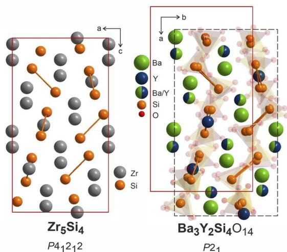
Fig. 10 Structure of  $\text{Zr}_5\text{Si}_4$  ( $P4_12_12$ ),<sup>64</sup> left, compared to  $\text{Ba}_3\text{Y}_2[\text{Si}_2\text{O}_7]_2$  refined in  $P2_1$ , right. Disilicate groups are shown with partial transparency to emphasize the Ba–Y–Si network. The pairs of silicon atoms corresponding to disilicate groups are linked.
