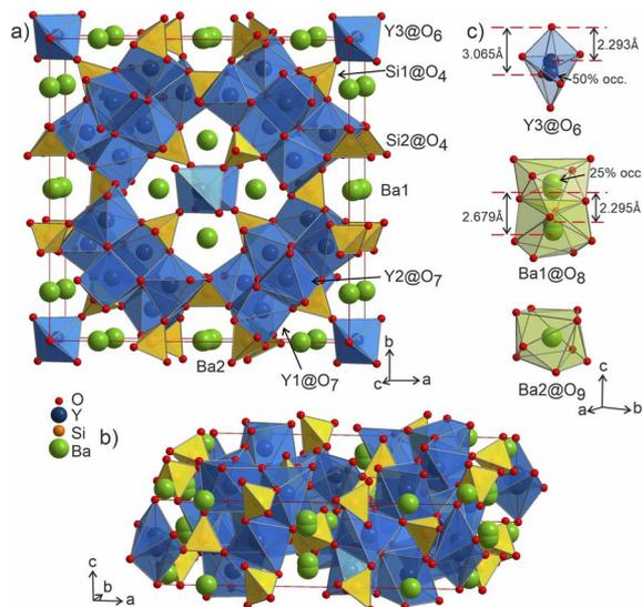
Fig. 3 (a and b) Structure of phase A  $\text{Ba}_5\text{Y}_{13}[\text{SiO}_4]_8\text{O}_{8.5}$  with silica tetrahedra and yttrium-centred polyhedra drawn in yellow and blue, respectively. (c) The Ba1 and Ba2-centred polyhedra (green shading) drawn oriented along the  $c$  axis.  $\text{Y3@O}_6$  octahedron is shown along the same direction, shaded in a light-blue colour to provide a better view on disordered atomic site.
