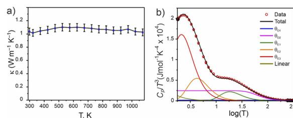
Fig. 11 Physical properties of  $\text{Ba}_5\text{Y}_{13}[\text{SiO}_4]_8\text{O}_{8.5}$ . (a) Thermal conductivity measured from 300 to 1073 K. (b) Heat capacity modelled as  $C_p/T^3(\log T)$  through a combination of two Debye, three Einstein, and one linear term (Table S15†).
