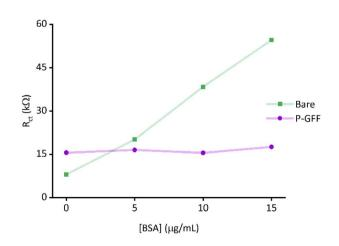
Fig. 7 Extracted  $R_{\rm ct}$  parameters for BSA incubation of both bare and P-GFF modified Au-SPEs.
