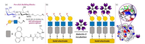
Fig. 1 An overview of the GFF-biosensor for galectin-3 detection. (a) The chemical structures and schematic representations of the core building blocks of the sensor: glycofluoroform Gal3F- $\beta$ (1,3)-GlcNAc-N<sub>3</sub> and polymeric thiol linker DBCO-(PHEA)<sub>25</sub>-SH. (b) Schematic diagram of the assembled biosensor and the proposed galectin-3 binding interaction. (c) Binding of an analogous native glycoform, LacNAc, on the surface of galectin-3 (PDB: 1KJL).<sup>34</sup>
