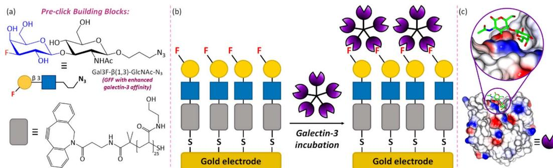
Fig. 1 An overview of the GFF-biosensor for galectin-3 detection. (a) The chemical structures and schematic representations of the core building blocks of the sensor: glycofluoroform Gal3F- $\beta$ (1,3)-GlcNAc- $N_3$  and polymeric thiol linker DBCO-(PHEA)<sub>25</sub>-SH. (b) Schematic diagram of the assembled biosensor and the proposed galectin-3 binding interaction. (c) Binding of an analogous native glycoform, LacNAc, on the surface of galectin-3 (PDB: 1KJL).<sup>34</sup>
