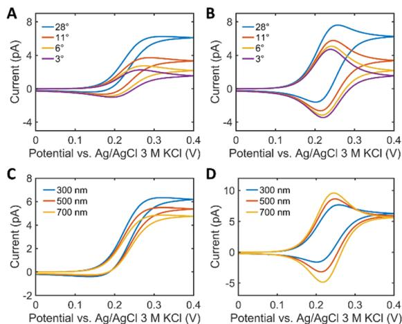
Fig. 3 The effect of the tip slope and the droplet thickness on the voltammograms. (A and B) SECCM voltammogram of 1 mM  $\text{Fc}(\text{MeOH})_2$  with the semi-angle ( $\theta$ ) of 3°, 6°, 11°, and 28° at a WF of (A) 1.2 and (B) 5. (C and D) SECCM voltammogram of 1 mM  $\text{Fc}(\text{MeOH})_2$  with the  $\theta$  of 28° as a function of the droplet thickness ( $h$ ) when the WF is (C) 1.2 and (D) 5.
