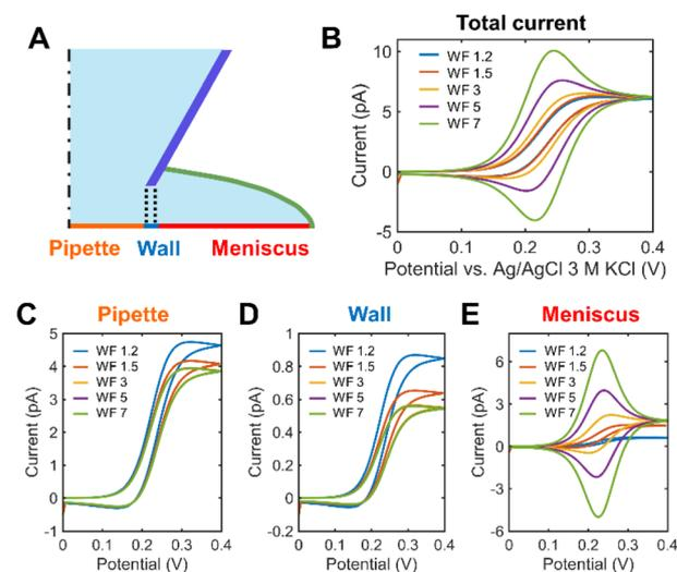
Fig. 2 SECCM voltammograms depending on the droplet diameter ( $d_{\text{drp}}$ ) while the tip diameter ( $d_{\text{tip}}$ ) is fixed to 900 nm. (A) The electrode surface was divided into three areas according to the types of the dominant mass transport flux. (B) Overall voltammogram of 1 mM Fc(MeOH)<sub>2</sub> with a scan rate of 1 V s<sup>-1</sup> in dependence of the wetting factor (WF). (C–E) The contribution of (C) pipette, (D) wall, and (E) meniscus parts to the overall voltammogram.
