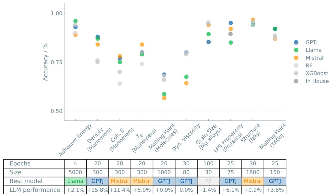
Fig. 1 Overview of the “Materials and properties” case studies. The accuracies of binary classifiers are plotted for the “Materials and properties” case studies. Three different LLMs (GPT-J, Llama, and Mistral) and two traditional ML models (random forest (RF) and XGBoost) are compared. The dashed line indicates the zero-rule baseline of 50% accuracy. The table summarizes the number of epochs (for fine-tuning the LLMs), training set size, the best-performing model, and the relative difference between the best LLM and the best “traditional” model.
