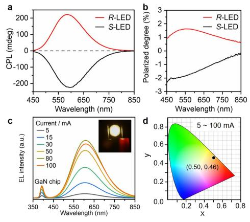
Fig. 5 (a) CPL spectra of *R/S*-LEDs fabricated by encapsulating *R/S*-2C polycrystals onto a 365 nm ultraviolet GaN LED chip. (b) Polarized degree of the *R/S*-LED devices. The CPL characterization of the LED devices powered by 3.0 V. (c) EL spectra and (d) chromaticity coordinates of the *R*-LED at different driving currents (5–100 mA). Inset of (c): photographs of the fabricated LEDs under operation.
