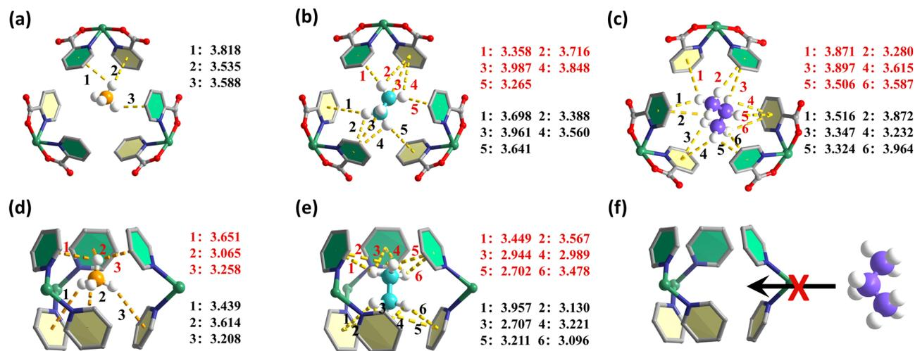
Fig. 4 GCMC simulated adsorption binding sites for (a)  $\text{CH}_4$ , (b)  $\text{C}_2\text{H}_6$  and (c)  $\text{C}_3\text{H}_8$  in nanotrap 1, (d)  $\text{CH}_4$  and (e)  $\text{C}_2\text{H}_6$  in nanotrap 2 and (f) the size limitation of nanotrap 2 for  $\text{C}_3\text{H}_8$ . The unit of interaction distance is angstrom ( $\text{\AA}$ ).
