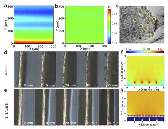
Fig. 4 SECM feedback images of (a) bare Zn and (b) Bi SAs@Zn anodes after zinc deposition for 600 s at 5 mA cm $^{-2}$ . (c) TEM image of Bi SAs@Zn after zinc deposition for 600 s at 5 mA cm $^{-2}$ . In situ optical microscope images of (d) bare Zn and (e) Bi SAs@Zn electrodes during Zn plating at 5 mA cm $^{-2}$ . COMSOL electric field simulation of (f) bare Zn and (q) Bi SAs@Zn.
