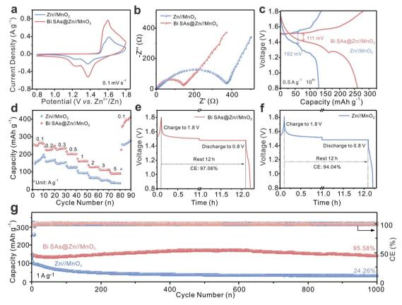
Fig. 5 (a) CV curves at a scan rate of  $0.1 \text{ mV s}^{-1}$ , (b) EIS plots before cycling, (c) charge/discharge profiles at the  $10^{\text{th}}$  cycle with a current density of  $0.5 \text{ A g}^{-1}$ , and (d) rate performance of Bi SAs@Zn//MnO<sub>2</sub> and Zn//MnO<sub>2</sub> full cells. Self-discharging voltage—time curves of (e) Bi SAs@Zn and (f) bare Zn. (g) Cycling performance of Zn//MnO<sub>2</sub> and Bi SAs@Zn//MnO<sub>2</sub> full cells at  $1 \text{ A g}^{-1}$ .
