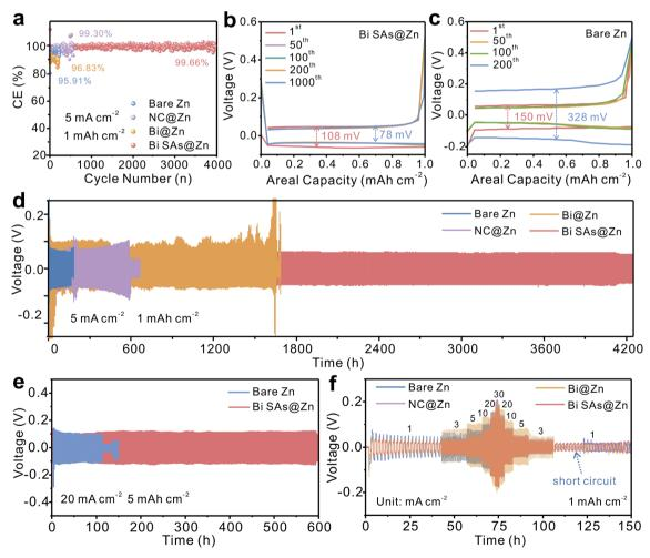
Fig. 3 (a) CE profiles of Zn//Ti, NC@Zn//Ti and Bi SAs@Zn//Ti at 5 mA cm $^{-2}$  and 1 mAh cm $^{-2}$ . Galvanostatic charge/discharge curves of (b) Bi SAs@Zn//Ti and (c) Zn//Ti. (d) Long-term cycling stability of bare Zn, NC@Zn, Bi@Zn, and Bi SAs@Zn symmetric cells at 5 mA cm $^{-2}$  and 1 mAh cm $^{-2}$ . (e) Cycling stability at 20 mA cm $^{-2}$  and 5 mAh cm $^{-2}$  and (f) rate performance at different current densities from 1 to 30 mA cm $^{-2}$  of bare Zn and Bi SAs@Zn.
