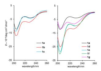
Fig. 5 Electronic circular dichroism (ECD) spectra of 1a-1g. Data were recorded at a peptide concentration of  $61 \mu M$  in  $CF_3CH_2OH$ .
