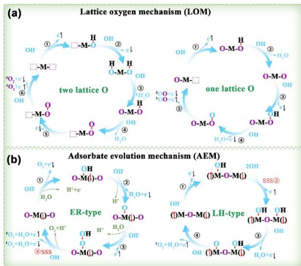
Fig. 10 (a) LOM and (b) AEM of OER examined by taking into account the spin of the transferred electrons.<sup>95</sup> M denotes the metal site, with the adjacent arrow indicating the spin direction of unpaired  $t_{2g}$  electrons. Purple O and blue O represent the lattice and adsorbed O species, respectively. SSS stands for the spin selective step.
