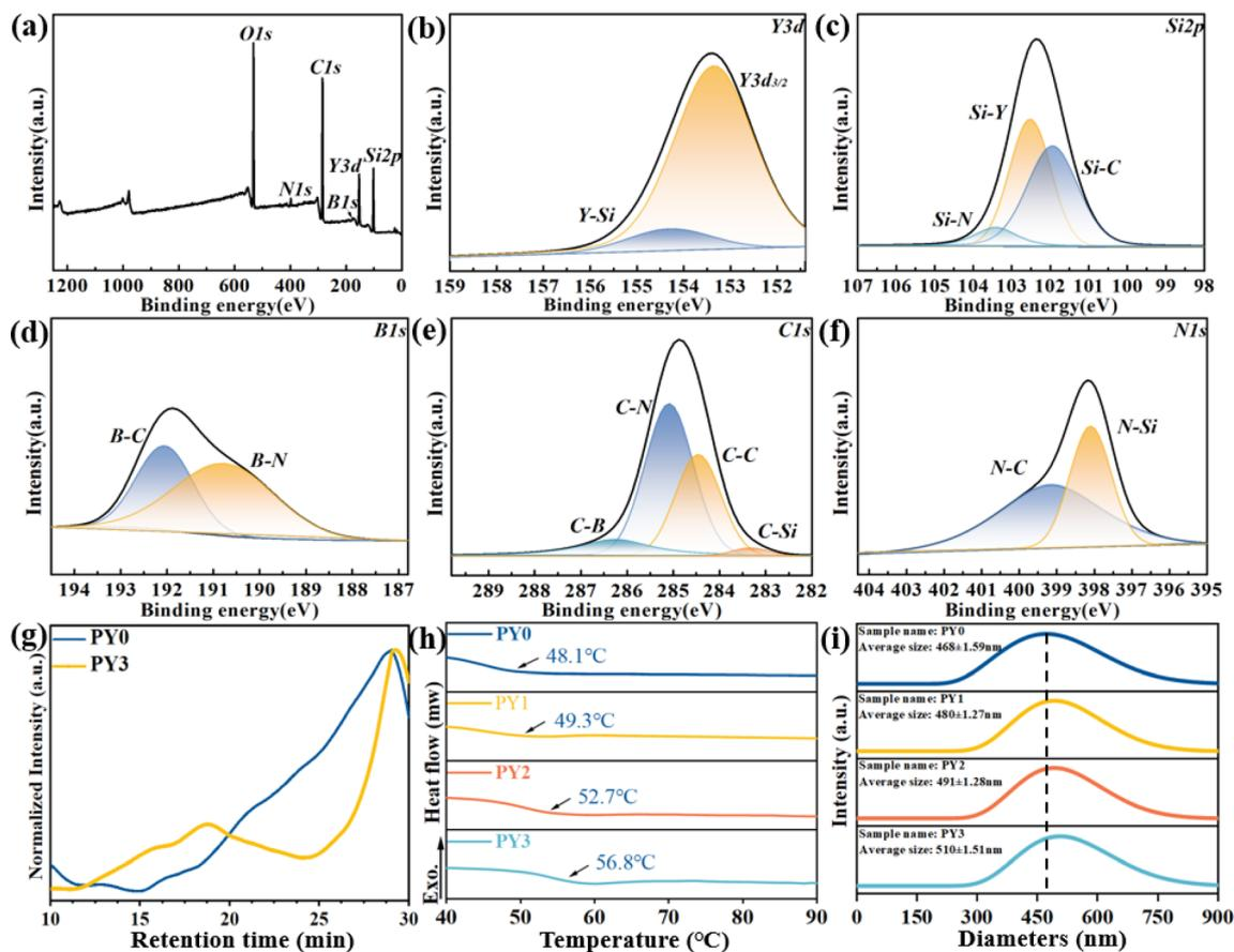
Fig. 2 (a) Full spectrum, (b) Y 3d peaks, (c) Si 2p peaks, (d) B 1s peaks, (e) C 1s peaks, and (f) N 1s peaks of the PY3 sample. (g) GPC curve, (h) DSC curve ( $N_2$  atmosphere, heating rate:  $2\text{ }^\circ\text{C min}^{-1}$ ), and (i) particle size distribution of PY0–PY3.
