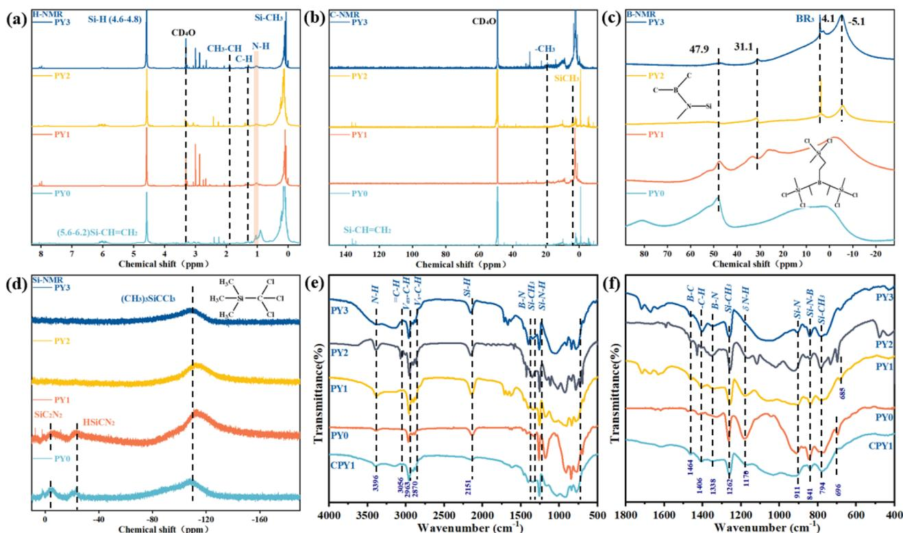
Fig. 1 The (a)  $^1\text{H}$  NMR spectrum, (b)  $^{13}\text{C}$  NMR spectrum, (c)  $^{11}\text{B}$  NMR spectrum, (d)  $^{29}\text{Si}$  NMR spectrum. (e and f) FT-IR spectra of PY0–PY3.
