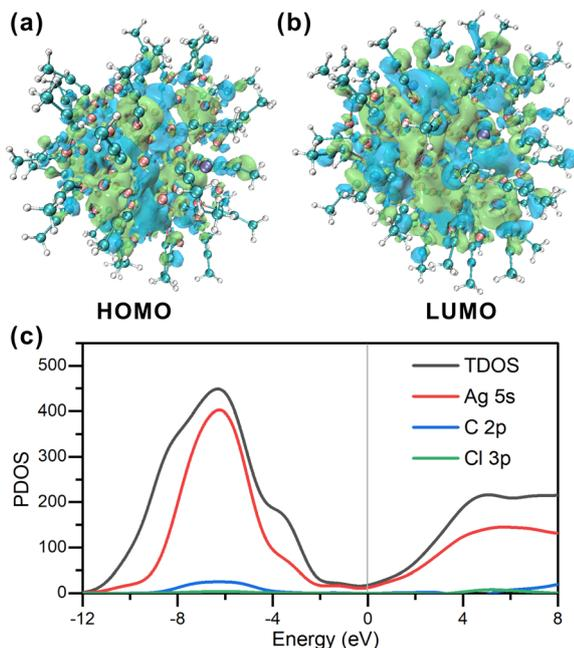
Fig. 5 (a and b) Frontier orbitals of  $\text{Ag}_{98}$ . (c) PDOS of  $\text{Ag}_{98}$ . The HOMO levels are positioned at the zero-energy level.
