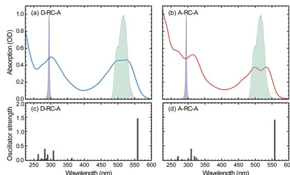
Fig. 1 (a and b) Static UV/visible absorption spectra of D-RC-A ((a), blue) and A-RC-A ((b), red) in THF solution ( $10^{-5}$   $\text{mol L}^{-1}$ ), overlapped with spectra of UV (violet shaded) and visible (green shaded) excitation pulses employed in the fs-TA experiments. (c and d) TD-DFT-calculated vertical excitation energies and oscillator strengths of D-RC-A (c) and A-RC-A (d).
