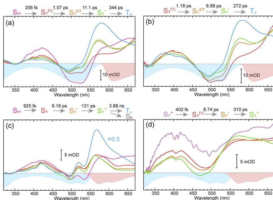
Fig. 3 Target-analysis-extracted species-associated spectra (SAS) of  $\lambda_{\text{ex}}$ -dependent fs-TA signals of D-RC-A upon 295 nm UV (a) and 513 nm visible (b) optical excitation, as well as SAS of A-RC-A upon identical UV (c) and visible (d) excitation. Four or five independent species were employed to reproduce the fs-TA signals.
