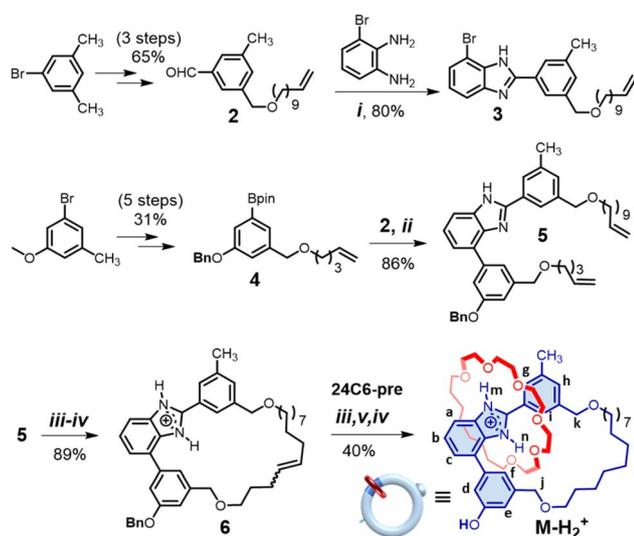
**Scheme 1** Synthesis of the hydroxyl [2]catenane  $[M-H_2][BF_4]$ . Conditions: (i)  $ZrCl_4$ ,  $CHCl_3$ , 25 °C, 24 h; (ii)  $Pd(Ph_3P)_4$ , 2 M  $Na_2CO_3$ , THF, 80 °C, 4 h; (iii) Grubbs' catalyst,  $CH_2Cl_2$ , 43 °C, 24 h; (iv)  $HBF_4$ , 30 min; (v)  $H_2$ , Pd/C, 25 °C, 4 h.
