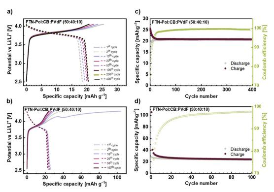
Fig. 6 (a) and (b) Galvanostatic charge and discharge profiles of selected cycles with a current density of 100 mA h g $^{-1}$  for different voltage ranges +2.5 to +4.0 V and +2.5 to +4.3 V. (c) and (d) Constant current cyclings at 100 mA h g $^{-1}$  for 100 and 400 cycles. Normalisation is with respect to active material FTN and FTN-Pol. In (c) and (d), capacity of CB was subtracted.
