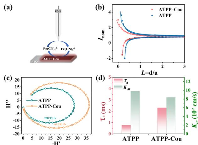
Fig. 4 (a) Schematic illustration of the testing process using SPECM. (b) Probe approach curves of ATPP and ATPP–Cou. (c) IMPS response curves recorded in PBS solution. (d)  $\tau_d$  and  $K_{eff}$  values of ATPP and ATPP–Cou.
