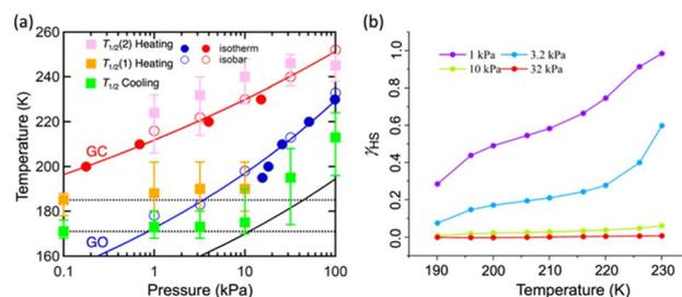
Fig. 5 (a) Correlation of the gated  $\text{CO}_2$  sorption behaviour with the SCO transition temperatures of framework **1** under variable  $\text{CO}_2$  pressures in the temperature range of 160–260 K; (b) HS fraction population ( $\gamma_{\text{HS}}$ ) of **1** under variable  $\text{CO}_2$  pressures ( $P_{\text{CO}_2} = 1$  to 32 kPa) in the temperature range of 190–230 K.
