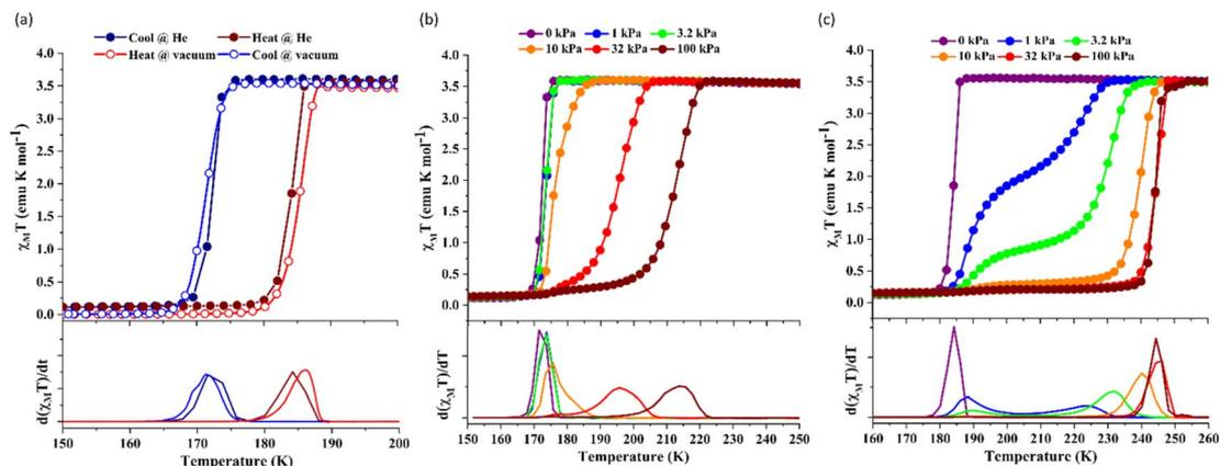
Fig. 4 Variation of the magnetic properties of framework **1** under  $\text{CO}_2$  adsorption under  $H_{\text{dc}} = 1$  kOe. (a) Magnetic susceptibility plots in the absence of any gas (open circles) and under 100 kPa He gas (filled circles). (b) The  $\text{CO}_2$  pressure dependence of the magnetic susceptibility measurements in cooling and (c) heating mode. First derivative plots are displayed at the bottom.
