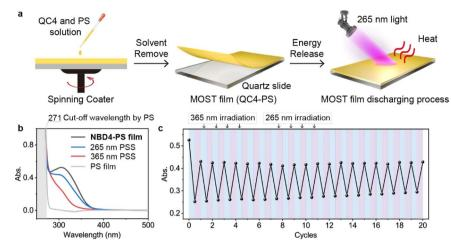
Fig. 6 Two-way photo-switching system in a MOST film. (a) Fabrication of a MOST film. (b) UV-Vis absorption spectra of the NBD4-PS film at the 365 nm PSS and the 265 nm PSS. (c) Two-way photoswitching cycling test of the NBD4-PS film.
