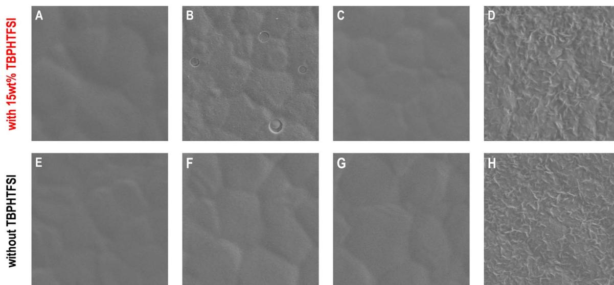
Fig. 4 Top-view scanning electron microscopy images of the organic semiconductor–TBPHTFSI composite layers deposited on the surface of FAPbI<sub>3</sub> perovskite polycrystalline thin films and the corresponding pristine organic semiconductor layers: (A and E) spiro-OMeTAD, (B and F) p-DTPF4, (C and G) p-DTPF4-EBEH, (D and H) p-EBEH. Image size: 5 μm × 5 μm. Encapsulation materials and gold electrodes were removed before imaging.
