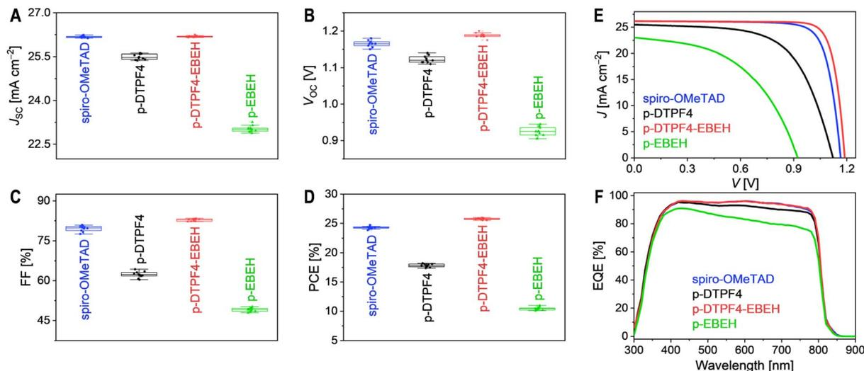
Fig. 3 (A–D) Statistical analysis of photovoltaic parameters of PSCs fabricated with varying hole transport layers under simulated AM1.5G irradiation at  $100 \text{ mW cm}^{-2}$ : (A) short-circuit photocurrent density ( $J_{sc}$ ); (B) open-circuit voltage ( $V_{oc}$ ); (C) fill factor (FF); (D) power conversion efficiency (PCE). (E) Representative photocurrent density–voltage ( $J$ – $V$ ) curves. (F) External quantum efficiency (EQE) spectra.
