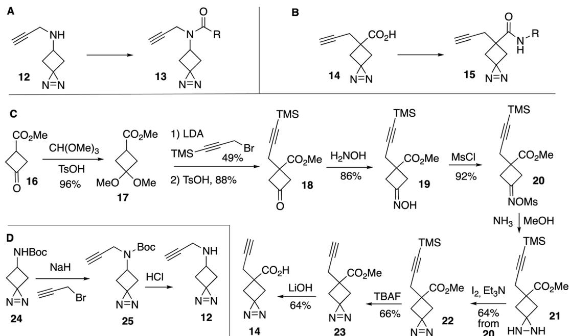
Fig. 3 Synthesis of alkyne-functionalized cyclobutanediazirines. Probes based on (A) *N*-(propynyl)-1,2-diazaspiro[2.3]hex-1-ene-5-amine and (B) 5-propynyl-1,2-diazaspiro[2.3]hex-1-ene-5-carboxylic acid. (C) Synthesis of **14**. (D) Synthesis of **12** and **24**.
