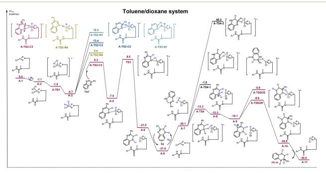
Scheme 6 DFT calculated energy potential surface for the proposed pathway in toluene/dioxane systems. (Ar = 3,5-di-CF<sub>3</sub>Ph; the phenyl groups on the phosphorus atoms are omitted for clarity; the relative Gibbs energies are labelled in kcal mol<sup>-1</sup>).
