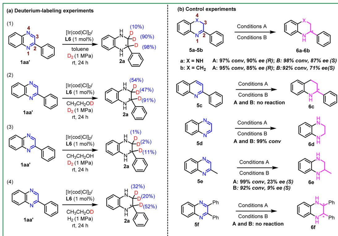
**Scheme 4** (a) Deuterium-labeling experiments of **1aa'**; (b) control experiments of various N-heteroaromatic compounds. Conditions A; substrate/[Ir(cod)Cl]<sub>2</sub>/L6 = 100/0.5/1 in 2 mL toluene/dioxane = 4 : 1, room temperature, 18 h and 2 MPa H<sub>2</sub>. Conditions B; substrate/[Ir(cod)Cl]<sub>2</sub>/L6 = 100/0.5/1 in 2 mL EtOH, room temperature, 18 h and 2 MPa H<sub>2</sub>. Yields were all isolated yields. The ee values were determined by HPLC.
