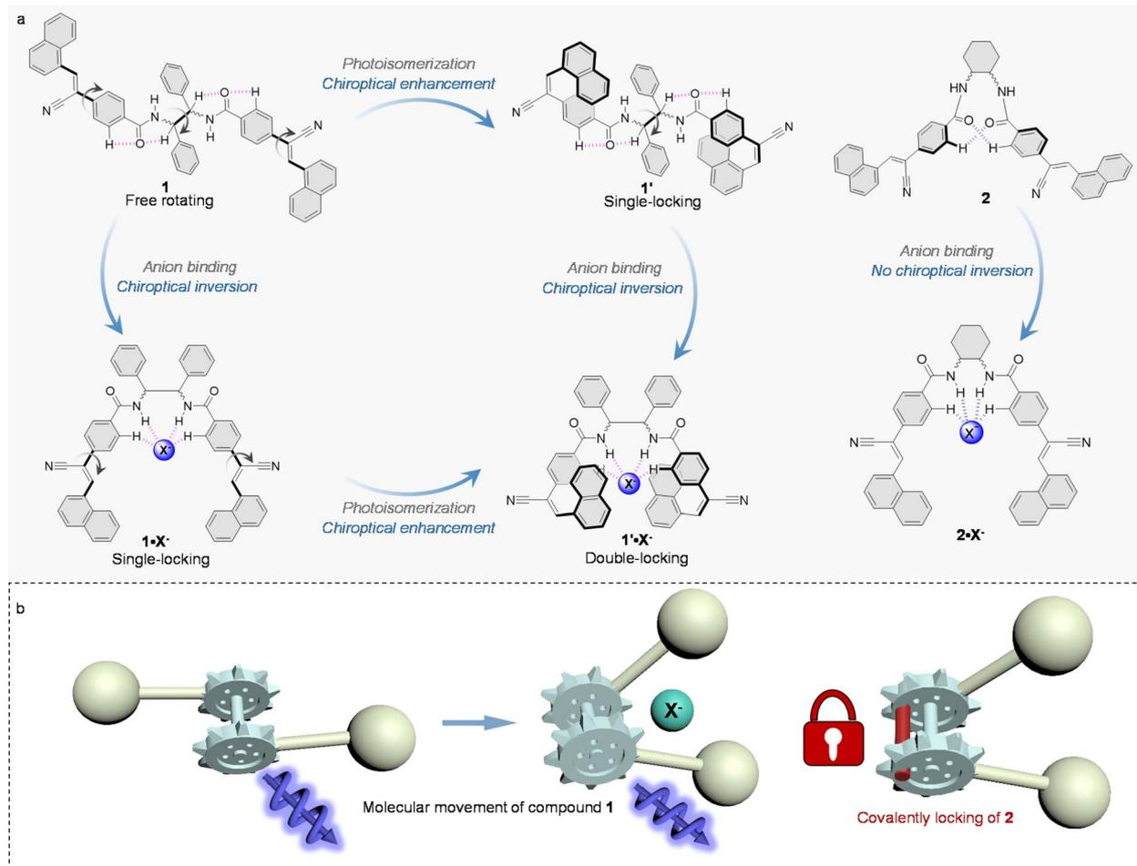
Scheme 1 (a) Transformation of the structure and properties of compound **1** and reference compound **2** by photoisomerization and anion binding. (b) Schematic representation of the chiroptical molecular movement invoked by anion binding.
