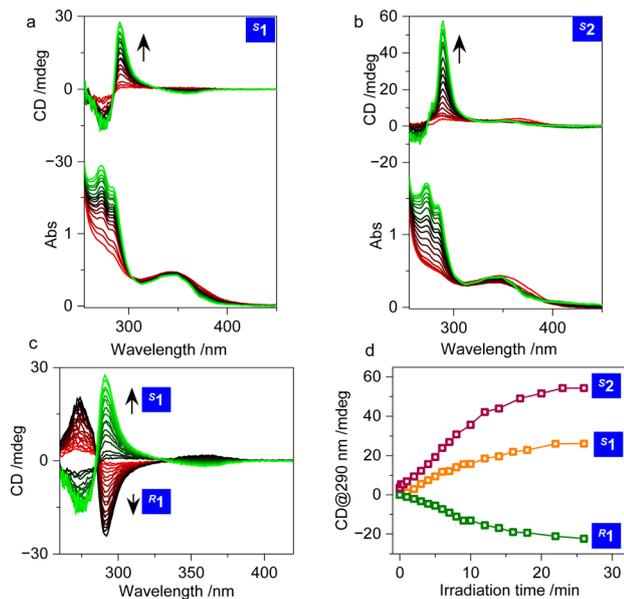
Fig. 2 (a–c) CD spectra of compounds **1** and **2** in DMSO under irradiation with 365 nm UV light (0.1 mM). (d) Cotton effect intensity at 290 nm for  $R_1$ ,  $S_1$  and  $S_2$  as a function of photo irradiation time.
