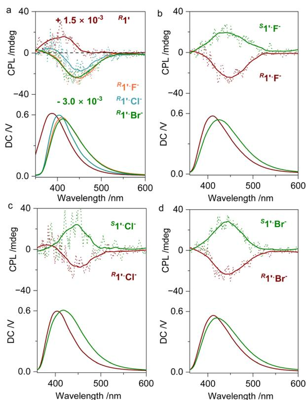
Fig. 5 CPL spectra of the systems after irradiation at 365 nm for 10 min. (a) Comparison of  $R^1$ ,  $R^1F^-$ ,  $R^1Cl^-$  and  $R^1Br^-$  (0.1 mM, 1 : 1 in THF). (b–d) CPL spectra of  $R^1/S^1X^-$  ( $X^- = F^-, Cl^-, Br^-$ ), ( $\lambda_{\text{ex}} = 340$  nm).
