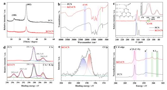
Fig. 2 (a) Powder XRD patterns, (b) FT-IR spectra, (c) solid-state <sup>13</sup>C NMR spectra (inset: normalization intensity of solid-state <sup>13</sup>C NMR spectra) and (d) C 1s XPS spectra of PCN and KCl-CN; (e) Cl 2p spectrum of KCl-CN; (f) C K-edge XANES curves of PCN and KCl-CN.
