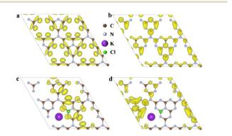
Fig. 1 The highest occupied molecular orbital (HOMO) and lowest unoccupied molecular orbital (LUMO) distributions in PCN (a and b), and K<sup>+</sup>, Cl<sup>-</sup> co-doped CN (c and d), respectively.
