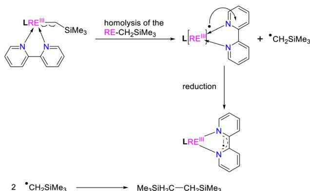
Scheme 13 Proposed homolytic redox reaction (HRR) for the generation of the bipyridyl radical anion.
