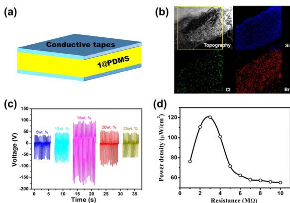
Fig. 5 Construction and performance of the PEG. (a) Schematic diagram of the PEG. (b) Cross-sectional scanning electron microscopy (SEM) and mapping images of 15 wt% 1@PDMS. (c)  $V_{\text{oc}}$  for 1@PDMS with different mass fractions with thumb pressure. (d) Power density as a function of load resistance for 15 wt% 1@PDMS.
