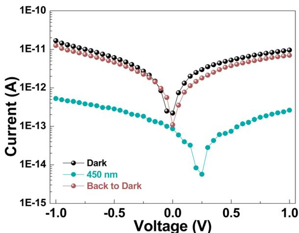
Fig. 5 Current–voltage ( $I$ – $V$ ) plots of (TMA)AgBr<sub>2</sub> in the dark and under the influence of 450 nm laser irradiation.
