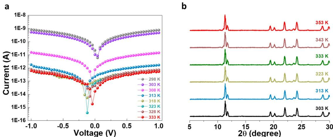
Fig. 4 Metallic conduction without structural change. (a) Variable-temperature current–voltage ( $I$ – $V$ ) diagram of (TMA)AgBr<sub>2</sub> in the temperature range from 298 K to 333 K, illustrating thermally deactivated charge transport. (b) Variable temperature PXRD patterns showing the retention of the structural phase over the temperature range.
