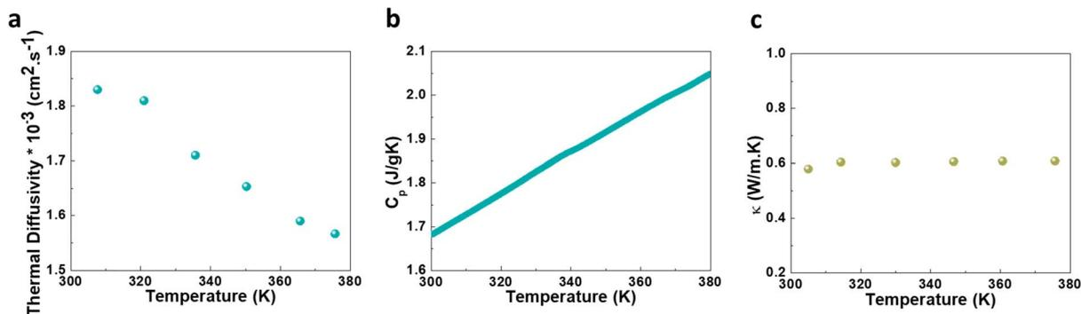
Fig. 3 Possibility of electron-phonon coupling. (a) Thermal diffusivity of (TMA)AgBr<sub>2</sub> as a function of temperature. (b) Heat capacity ( $C_p$ ) of (TMA)AgBr<sub>2</sub> as a function of temperature. (c) Variable temperature thermal conductivity of (TMA)AgBr<sub>2</sub> yielding an ultra-low value.
