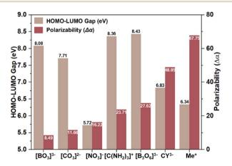
Fig. 1 Calculated HOMO–LUMO gaps and polarizability  $(\Delta\alpha)$  for inorganic and organic coplanar BAGs. Inorganic:  $[BO_3]^{3-},\ [CO_3]^{2-},\ [NO_3]^-,\ and\ [B_3O_6]^{3-}.$  Organic:  $[C(NH_2)_3]^+,\ [C_3N_6H_7]^+$  (Me<sup>+</sup>), and  $[C_3N_3O_3]^{3-}$  (CY $^{3-}$ ).
