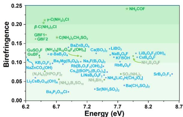
Fig. 5 Birefringence of selected DUV metal-free (green), metal-containing optical crystals (blue), along with results from this work (star). Details are listed in Table S8.<sup>†</sup>
