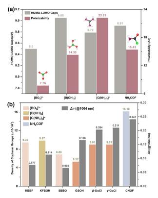
Fig. 4 (a) Calculated HOMO–LUMO gaps and polarizability for coplanar groups. (b) Density of coplanar groups and calculated birefringence (@1064 nm) in KBBF, KFBOH, SBBO,  $C(NH_2)_3CH_3SO_3$  (GSOH),  $\beta/\gamma-C(NH_2)_3Cl$  (GuCl), and  $NH_2COF$  (CNOF).
