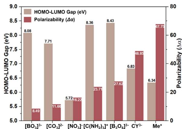
Fig. 1 Calculated HOMO–LUMO gaps and polarizability ( $\Delta\alpha$ ) for inorganic and organic coplanar BAGs. Inorganic:  $[\text{BO}_3]^{3-}$ ,  $[\text{CO}_3]^{2-}$ ,  $[\text{NO}_3]^-$ , and  $[\text{B}_3\text{O}_6]^{3-}$ . Organic:  $[\text{C}(\text{NH}_2)_3]^+$ ,  $[\text{C}_3\text{N}_6\text{H}_7]^+$  ( $\text{Me}^+$ ), and  $[\text{C}_3\text{N}_3\text{O}_3]^{3-}$  ( $\text{C}\gamma^{3-}$ ).
