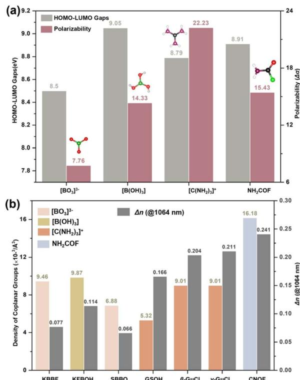
Fig. 4 (a) Calculated HOMO-LOMO gaps and polarizability for coplanar groups. (b) Density of coplanar groups and calculated birefringence (@1064 nm) in KBBF, KFBOH, SBBO,  $C(NH_2)_3CH_3SO_3$  (GSOH),  $\beta/\gamma-C(NH_2)_3Cl$  (GuCl), and  $NH_2COF$  (CNOF).
