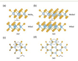
Fig. 1 Example  $2\times 2$  and  $3\times 3$  cluster models for the MoSe<sub>2</sub>-WSe<sub>2</sub> heterobilayer, with molybdenum atoms in light blue, tungsten atoms in darker blue, and selenium atoms in orange. Passivating hydrogens omitted for clarity. Black outline indicates one primitive cell.
