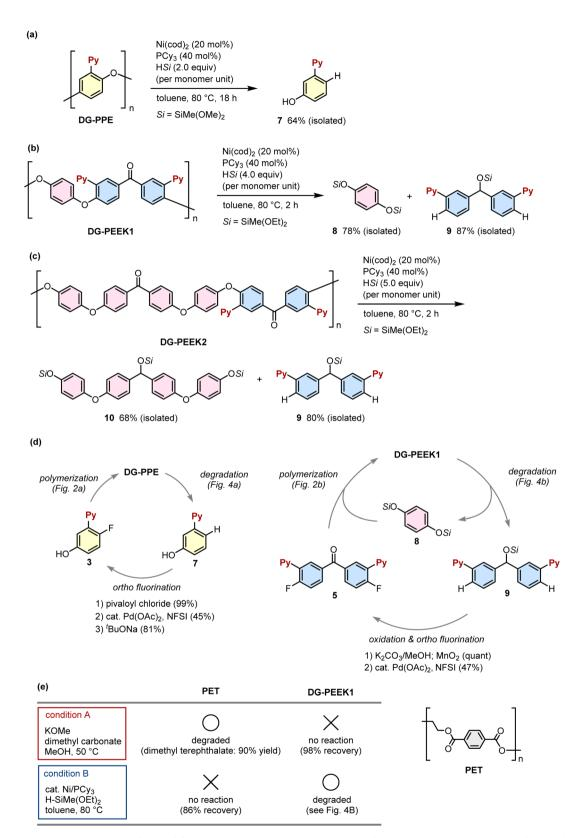
Fig. 4 (a) Controlled degradation of DG-PEEK2. (b) Controlled degradation of DG-PEEK1. (c) Controlled degradation of DG-PEEK2. (d) Chemical recycling of DG-PPE and DG-PEEK1. (e) Orthogonal degradation of PET and DG-PEEK1.
