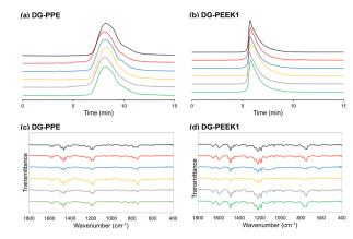
Fig. 3 Chemical stability of DG-PPE and DG-PEEK1.<sup>a</sup> SEC (a and b) and FT-IR (c and d) analysis measured after neutralization for polymer samples treated with the following solutions at rt for 24 h: black, none; red, HCl (12 M); blue, NaOH (10 M); orange, H<sub>2</sub>O<sub>2</sub> (30%); gray, AcOH; green, boiling water.
