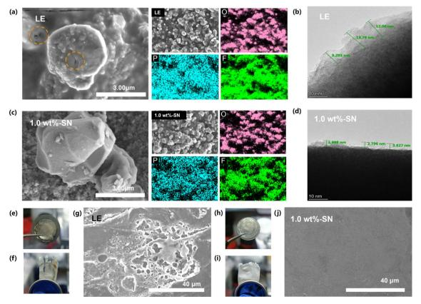
Fig. 4 SEM and EDS images of NCM811 cathodes after 100 cycles and TEM images of NCM811 cathodes after 20 cycles in (a, c) LE and (b, d) 1.0 wt%-SN. Lithium metal anode and diaphragm pictures and SEM images of lithium metal anodes after 20 cycles in (e, f, g) LE and (h, i, j) 1.0 wt%-SN.
