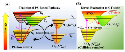
Scheme 1 Generation of  $O_2$  ( $a^1\Delta_q$ ) via (A) traditional PS-based approach and (B) direct excitation to the CT state
