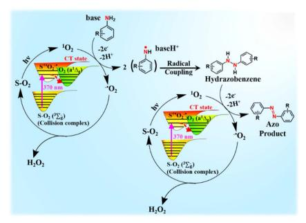
Scheme 4 Plausible reaction mechanism for the oxidative coupling of arylamines via PS-free singlet oxygen.
