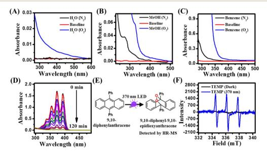
Fig. 1 UV-vis spectra of (A) water, (B) methanol, and (C) benzene under  $N_2$  and  $O_2$  atmosphere. (D) Changes in the absorption spectra of DPA in benzene under the irradiation of a 370 nm LED under an open atmosphere. (E) Schematic showing the conversion of DPA to 9,10-diphenyl-9,10-epidioxyanthracene under the irradiation of a 370 nm LED in benzene under an open atmosphere. (F) Changes in the EPR spectra of TEMP (50 mM) under dark and 370 nm LED irradiation for 30 min in aqueous medium.
