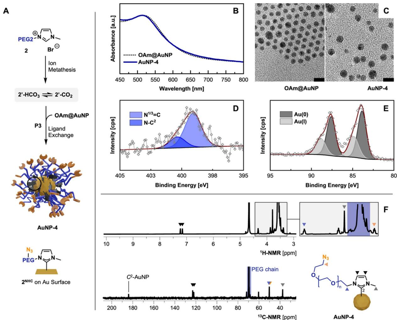
Fig. 3 (A) Optimized synthesis of AuNP-4 following P3; ion metathesis –  $\text{KHCO}_3$ , MeOH, 35 °C, 48 h; P3 THF, 40 °C, 62 h; characterization of AuNP-4 obtained via ligand exchange procedure P3: (B) UV-Vis comparison against OAm@AuNPs in THF; (C) TEM micrographs comparison (scale bar 10 nm); (D and E) high-res. XPS spectra of N 1s and Au 4f region; (F)  $^1\text{H}$ - and  $^{13}\text{C}$ -NMR (500 MHz,  $\text{D}_2\text{O}$ ) and structural assignment.
