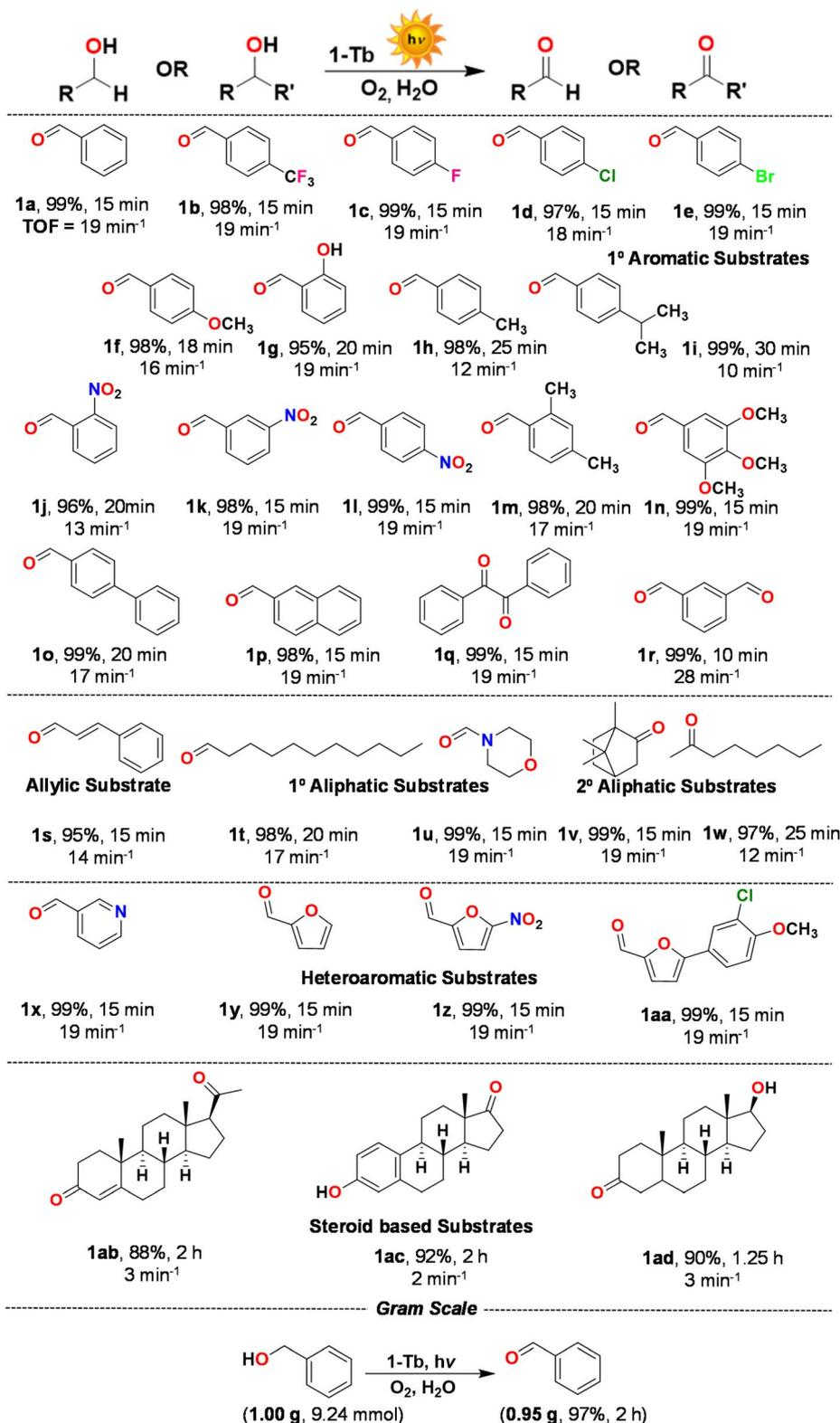
**Scheme 1** Substrate scope for the photocatalytic oxidation of assorted alcohols and a scale-up reaction. Reaction conditions: substrate (0.92 mmol), 1-Tb (1 mol%), H<sub>2</sub>O (2 mL), temperature (25 °C). All yields are for the isolated products. The characterization data and the corresponding spectra for the representative products are presented in Fig. S22–S84, ESI.†
