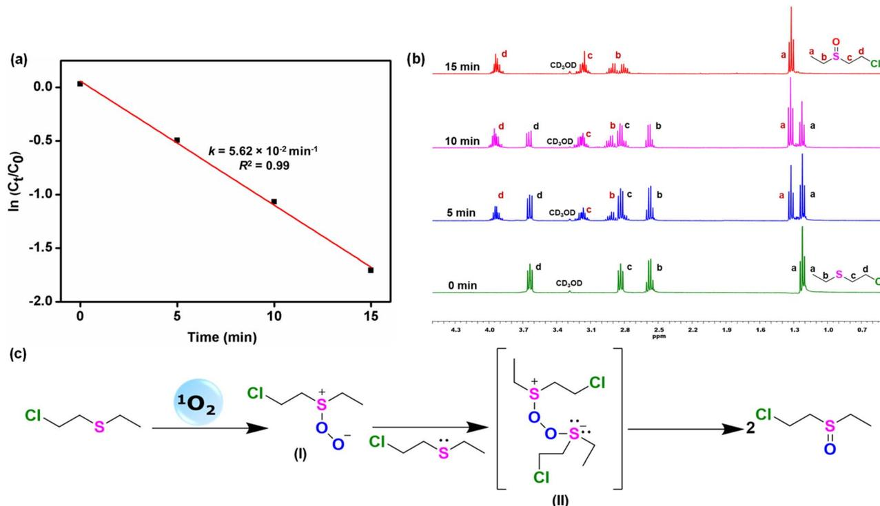
Fig. 4 (a) Plot of  $\ln(C_t/C_0)$  versus time representing first-order kinetics for the photo-oxidation of thioanisole in the presence of **1-Tb** as a photocatalyst. (b) Progress of the sulfoxidation reaction of CEES monitored by time-dependent  $^1\text{H}$  NMR spectra. (c) Proposed reaction mechanism for the selective oxidation of CEES using  $^1\text{O}_2$ .
