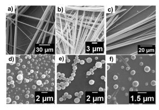
Fig. 6 SEM images of (a) 2, (b) 4 and (c) 5 showing their tubular morphology, and SEM images of (d) 6, (e) 7 and (f) 8 showing their spherical morphology. The samples were prepared by dissolving 1 mg of respective compounds in 1 mL of ACN.
