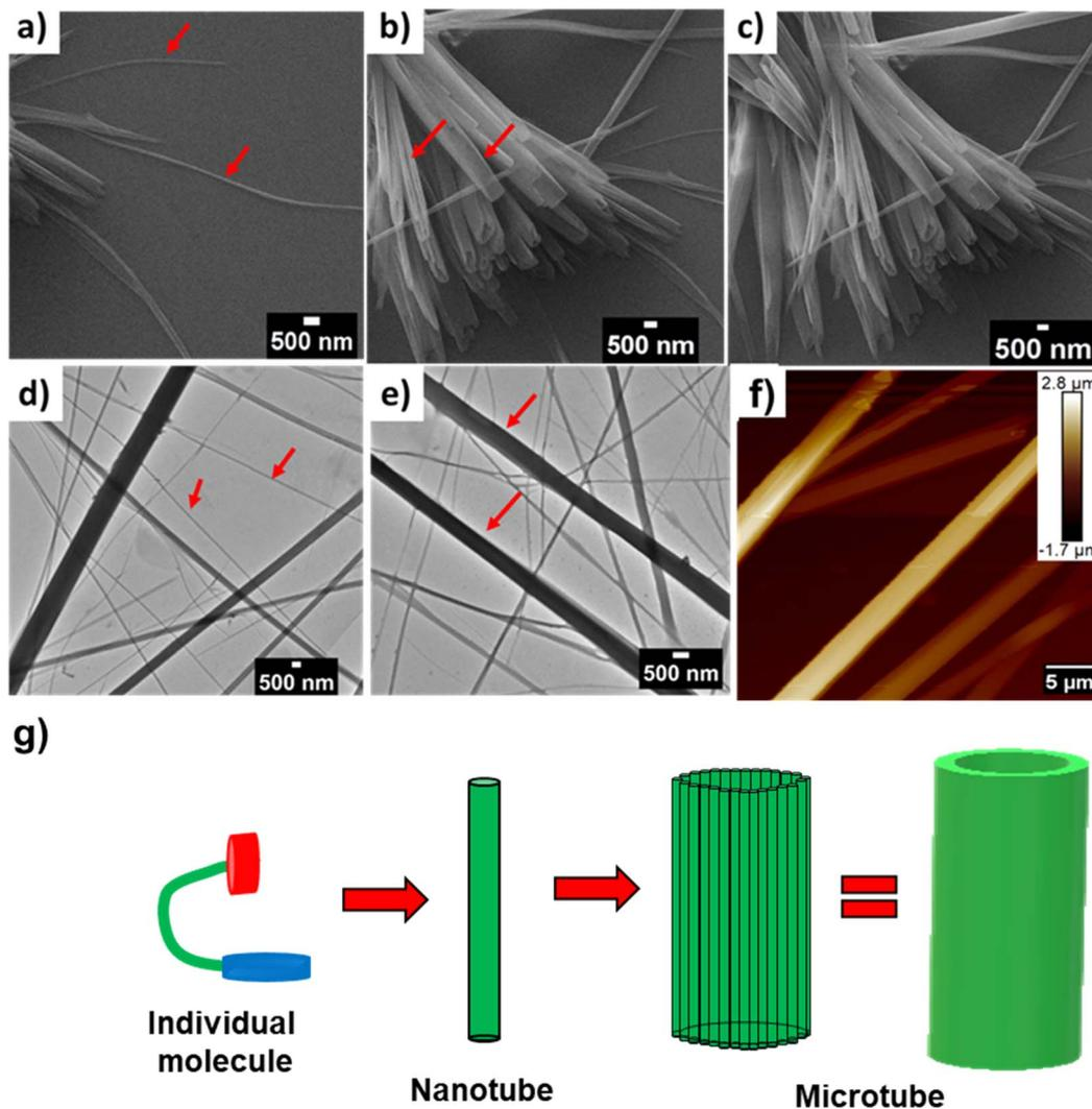
Fig. 4 SEM images of **1** show (a) tubular assembly (indicated by red arrows), (b) intermediate stage of microtube formation (marked by red arrows) and (c) microtube structure. TEM images of **1** show (d) tubular assembly (indicated by red arrows) and (e) microtube structure (indicated by red arrows). AFM image of **1** shows (f) microtubular assembly and (g) schematic representation of self-assembly of **1** to a microtube.
