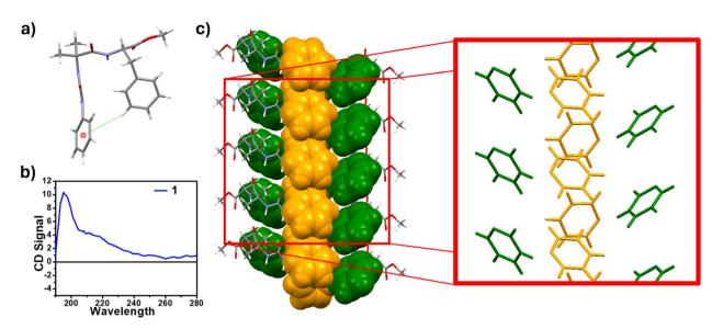
Fig. 2 (a) Crystal structure of peptide 1 showing the turn conformation. Intramolecular edge-to-face  $\pi - \pi$  interaction is shown as green dotted lines, (b) CD spectrum of peptide 1 in acetonitrile, (c) space-filling model of aromatic rings showing the Phe-Phe zipper arrangement. The zoomed-in part shows the orientation of aromatic rings.
