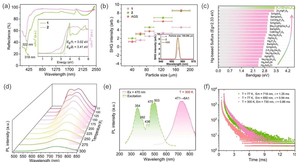
Fig. 3 (a) UV-vis diffuse reflection spectra of **1** and **2**; (b) phase-matchable behaviors of **1**, **2** and AGS with particle sizes of 150–200  $\mu\text{m}$ ; (c) bandgaps of typical Hg-based sulfurs with PM behavior ( $E_g > 2.33$  eV); (d) temperature-dependent (77–300 K) PL spectra of **1**; (e) PL excitation and emission spectra of **1** at room temperature; (f) PL decay lifetime curves of **1** recorded at 718 and 650 nm at 77 K.
