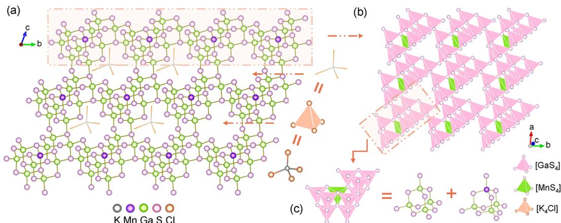
Fig. 1 (a) The ball-and-stick model of **1** viewed along the *a*-axis, accompanied by various morphologies of  $[K_4Cl]^{3+}$ -filled cations; (b) an independent 2D  $[MnGa_9S_{16}]^{3-}$  layered displayed as a polyhedron; (c) a basic repeating unit consisting of  $[Ga_4S_{10}]$  and  $[MnGa_3S_{10}]$  T2-supertetrahedra.
