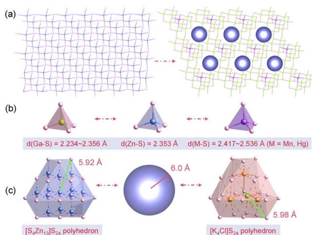
Fig. 2 (a) 3D wireframes of ZnS (left) and  $[MGa_9S_{16}]^{3-}$  (right); (b)  $[GaS_4]$ ,  $[ZnS_4]$ , and  $[MS_4]$  tetrahedra along with their range of bond lengths ( $M = Mn, Hg$ ); (c)  $[Zn_{13}S_4]S_{24}$  (left) and  $[K_4Cl]S_{24}$  (right) polyhedral modeling diagrams.
