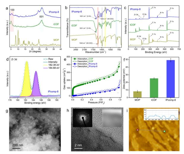
Fig. 2 (a) PXRD profile, (b) FTIR spectra, and (c) XPS survey spectra of IPcomp-8 along with the pristine materials, (d) deconvoluted Zr 3d XPS spectra of IPcomp-8, (e) N<sub>2</sub> sorption profile of iCOF and IPcomp-8 at 77 K, (f) comparison of zeta potential values of MOP, iCOF and IPcomp-8, (g) FESEM and (h) HRTEM images of IPcomp-8, (inset: lattice fringes and SAED images), and (i) AFM image and the corresponding height profile of IPcomp-8.
