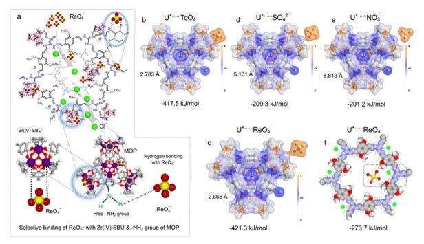
Fig. 5 (a) Illustration of mechanistic insight of selective  $ReO_4^-$  capture through different interactions by IPcomp-8. Density functional theory (DFT) calculations: (b-f) energy-optimized adsorption complexes for interactions between  $TcO_4^-$  or  $ReO_4^-$  with Zr(w)-SBU of the MOP and iCOF structural units with their corresponding binding energies.
