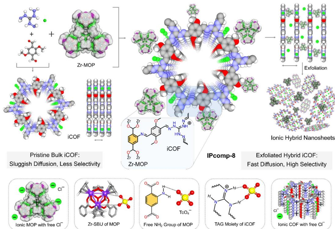
Fig. 1 Schematic representation of synthesis of an ultrathin hybrid composite material (IPcomp-8) by covalently embedding amino group functionalized Zr-MOP with iCOF and pristine iCOF. Various multifunctional features of IPcomp-8 showing ion-exchange electrostatic and functional group mediated interactions with radioactive oxoanions (color code: gray: carbon, white: hydrogen, red: oxygen, green: chlorine, light blue: nitrogen, violet: zirconium).
