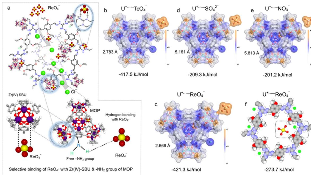
Fig. 5 (a) Illustration of mechanistic insight of selective  $\text{ReO}_4^-$  capture through different interactions by IPcomp-8. Density functional theory (DFT) calculations: (b–f) energy-optimized adsorption complexes for interactions between  $\text{TcO}_4^-$  or  $\text{ReO}_4^-$  with Zr(IV)-SBU of the MOP and iCOF structural units with their corresponding binding energies.
