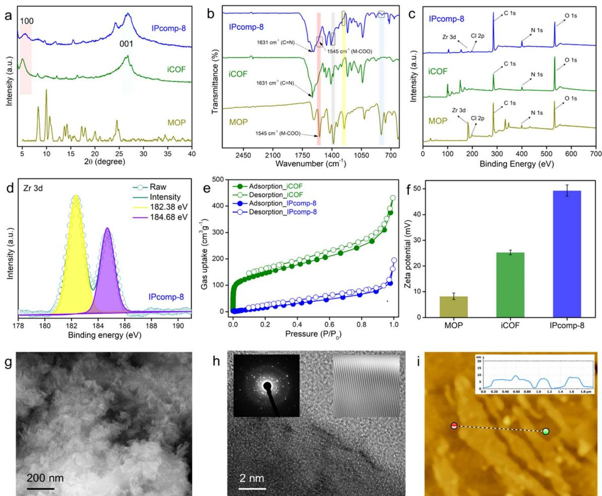
Fig. 2 (a) PXRD profile, (b) FTIR spectra, and (c) XPS survey spectra of IPcomp-8 along with the pristine materials, (d) deconvoluted Zr 3d XPS spectra of IPcomp-8, (e)  $N_2$  sorption profile of iCOF and IPcomp-8 at 77 K, (f) comparison of zeta potential values of MOP, iCOF and IPcomp-8, (g) FESEM and (h) HRTEM images of IPcomp-8, (inset: lattice fringes and SAED images), and (i) AFM image and the corresponding height profile of IPcomp-8.
