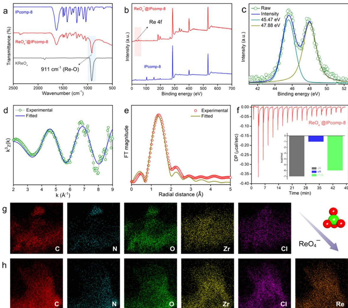
Fig. 4 (a) FT-IR spectra of  $\text{ReO}_4^-$  loaded IPcomp-8, (b) XPS survey spectra and (c) deconvoluted Re 4f core-level XPS spectra of IPcomp-8 and  $\text{ReO}_4^-$ @IPcomp-8, (d) raw and (e) Fourier transforms of Re L3 edge EXAFS spectra of  $\text{ReO}_4^-$  treated IPcomp-8, (f) ITC thermogram with its corresponding parameters, and (g and h) TEM EDX elemental mapping of IPcomp-8 and  $\text{ReO}_4^-$ @IPcomp-8, respectively.
