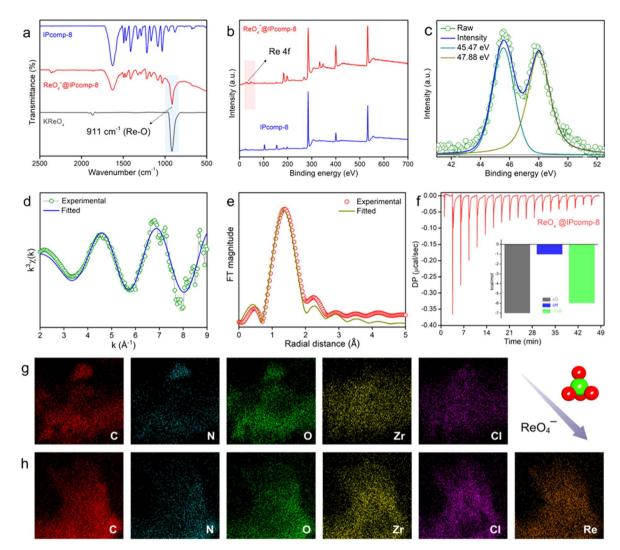
Fig. 4 (a) FT-IR spectra of  $ReO_4^-$  loaded IPcomp-8, (b) XPS survey spectra and (c) deconvoluted Re 4f core-level XPS spectra of IPcomp-8 and  $ReO_4^-$ @IPcomp-8, (d) raw and (e) Fourier transforms of Re L3 edge EXAFS spectra of  $ReO_4^-$  treated IPcomp-8, (f) ITC thermogram with its corresponding parameters, and (g and h) TEM EDX elemental mapping of IPcomp-8 and  $ReO_4^-$ @IPcomp-8, respectively.
