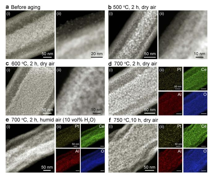
Fig. 3 (a–c) HAADF-STEM images of  $Pt@CeO_2/Al_2O_3$  (a) before and after aging in dry air at (b) 500 and (c) 600 °C for 2 h. (d–f) HAADF-STEM images and elemental mappings of  $Pt@CeO_2/Al_2O_3$  after aging (d) in dry air at 700 °C for 2 h, (e) in humid air (10 vol% of water) at 700 °C for 2 h, and (f) in dry air at 750 °C for 10 h.
