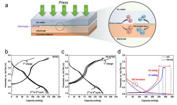
Fig. 2 (a) Schematic illustration of direct contact SCT. Charge–discharge profiles of  $Na_{0.67}Fe_{0.5}Mn_{0.5}O_2$  (b) before and (c) after sodium compensation. (d) Galvanostatic charge-discharge curves of HC electrodes with/without SCT. Reproduced with permission.<sup>30</sup> Copyright 2019, American Chemical Society.
