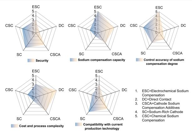
Fig. 10 Key parameter radar chart of different SCTs.
