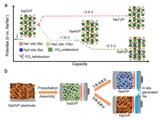
Fig. 8 (a) Schematic illustration for phase transformations of  $Na_xV_2(PO_4)_3$  and corresponding electrochemical potentials. (b) Illustration of sodium compensation on  $Na_xV_2(PO_4)_3$ , battery assembly, and battery operation within two different voltage windows. Reproduced with permission.<sup>81</sup> Copyright 2022, Wiley-VCH.
