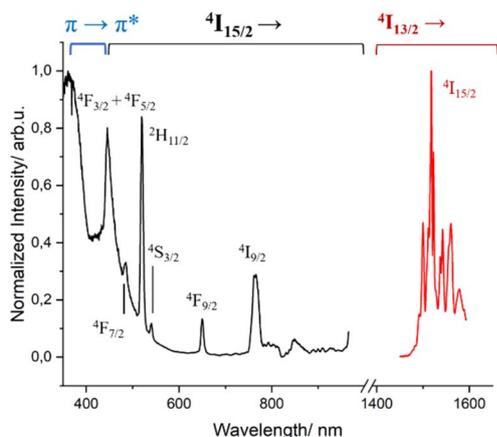
Fig. 4 Excitation ( $\lambda_{em} = 1530$  nm, black trace) and emission ( $\lambda_{exc} = 400$  nm, red trace) spectra of complex 2 in MeOH- $d_4$ : DMSO- $d_6$  (1 : 1) at 77 K.
