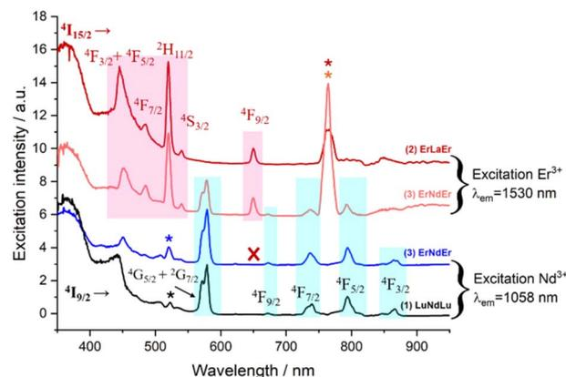
Fig. 8 Excitation spectra of complexes (1) at  $\lambda_{\text{em}} = 1058$  nm (black trace), (2) at  $\lambda_{\text{em}} = 1530$  nm (red trace) and (3) at  $\lambda_{\text{em}} = 1058$  nm (blue trace) and at  $\lambda_{\text{em}} = 1530$  nm (orange trace) in  $\text{MeOH-d}_4/\text{DMSO-d}_6$  (1 : 1) at 77 K.
