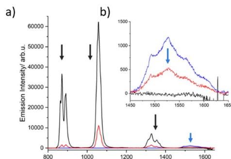
Fig. 6 Emission spectra ( $\lambda_{exc} = 400$  nm) of iso-absorbant solutions of complexes (1) (black trace), (2) (blue trace), and (3) (red trace) in MeOH- $d_4$ : DMSO- $d_6$  (1 : 1) solution at room temperature (a) with the corresponding  $Er^{3+}$  emission zoom (b).
