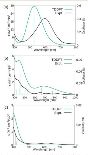
Fig. 8 Simulated and experimental (Et<sub>2</sub>O) UV-visible absorbance spectra of (a)  $(Cp_2^*Sc)_2(\mu-\eta^1:\eta^1-N_2)$ , 1, (b)  $Cp_2^*Sc[(\mu-\eta^2:\eta^2-N_2)ScCp_2^*]_2$ , and (c) the side-on isomer of 3,  $Cp_2^*Sc(\mu-\eta^2:\eta^2-N_2)ScCp^*|(THF)$ . A Gaussian spectral line shape with a width of 0.2 eV was employed in each case.
