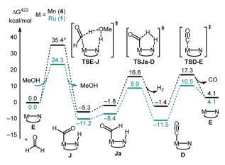
Fig. 5 Selected steps involved in the decarbonylation of formaldehyde using catalysts derived from 1 and 4 (PBE0-D3(BJ) $_{PCM(THF)}$ /def2-TZVP//RI-BP86 $_{PCM(THF)}$ /def2-SVP level). \*The structure of TSE-J does not contain protic assistance from MeOH for Mn-MACHO (4) as this was not found to stabilise the TS.
