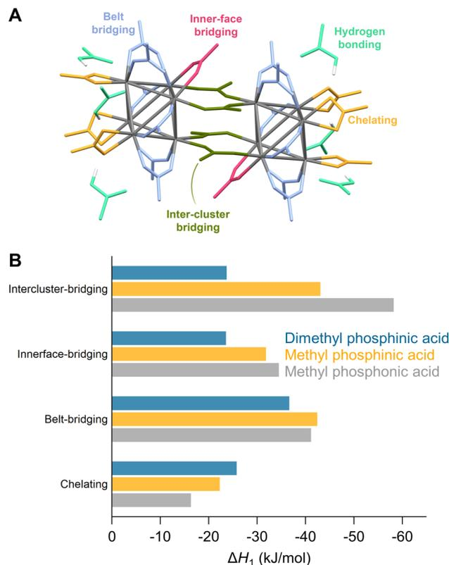
Fig. 3 (A) Different binding modes of acetate ligands in the structure of  $Zr_{12}O_{16}H_8(OOCMe)_{24} \cdot 6MeCOOH$  - CCDC-604528.<sup>5,17,55</sup> (B) Enthalpy of ligand exchange reactions at different binding sites.
