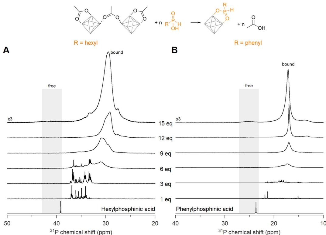
Fig. 5  $^{31}\text{P}$  NMR spectra of the titrations of **Zr12**-acetate with (A) hexyl- and (B) phenylphosphinic acid. The cluster concentration is  $20\text{ mg mL}^{-1}$  in  $\text{CDCl}_3$ .  $^{31}\text{P}$  NMR spectra of the free phosphinic acids with an equivalent of acetic acid are provided as references.
