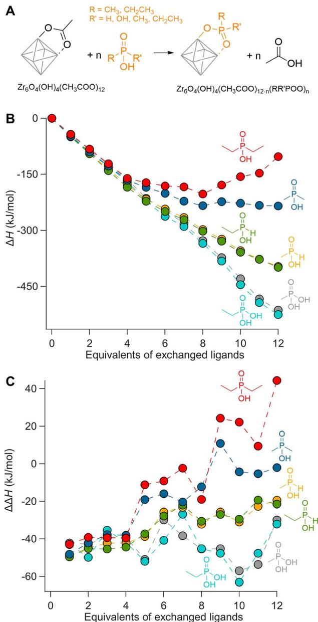
Fig. 1 (A) Scheme representing the exchange of acetate ligands for phosphorus-based ligands on a fully bridged **Zr6** cluster. (B) Enthalpy of ligand exchange reactions as a function of equivalents of exchanged ligands,  $\Delta H$ . (C) The enthalpy change for every step,  $\Delta\Delta H$ .
