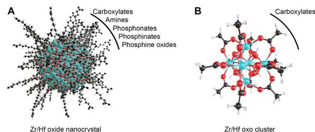
**Scheme 1** (A) Schematic representation of a colloidally stable zirconium/hafnium oxide nanocrystal depicting the inorganic core and organic ligand shell. (B) The structure of  $M_6O_8H_4(OOCR)_{12}$ , where the  $M_6O_8$  core is capped with four protons and twelve carboxylate ligands,  $M = Zr/Hf$ . The ligands that have been reported to cap nanocrystals and clusters in nonpolar media are listed. Cyan atoms represent zirconium or hafnium, all other atoms follow conventional CPK coloring.
