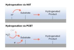
Fig. 4 Electricity-driven hydrogenation *via* hydrogen atom transfer (top) or proton-coupled electron transfer (bottom) processes.<sup>97</sup>
