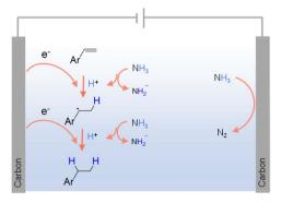
Fig. 3 Possible mechanism for the electrochemical hydrogenation of olefins using  $NH_3$  as the hydrogen source using  $0.1\,M$  LiClO<sub>4</sub> in CH<sub>3</sub>CN as the electrolyte with  $NH_3$  (1 atm) as the nitrogen source.<sup>83</sup>
