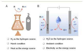
Fig. 1 General representations of (A) thermocatalytic hydrogenation using  $\rm H_2$  and (B) electrocatalytic hydrogenation using water as the hydrogen source.
