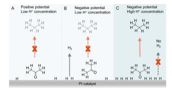
Fig. 10 Representations of acetone to propane hydrogenation (A) under positive potential in electrolyte with low H $^+$  (0.1 M H $_2$ SO $_4$ ) concentration, (B) under negative potential in electrolyte with low H $^+$  (0.1 M H $_2$ SO $_4$ ) concentration, and (C) under negative potential in electrolyte with high H $^+$  (1 M H $_2$ SO $_4$ ) concentration.
