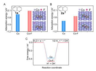
Fig. 8 (A and B) Comparisons of adsorption energies of 1a and 2a on pure Co (A) and Co-F (B), respectively (inset: the stable adsorption configurations of 1a and 2a). (C) The calculated free energy for H\* formation on Co versus CoF. This figure has been adapted/reproduced from ref. 112 with permission from Nature Publishing Group, copyright
