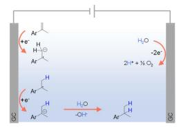
Fig. 5 Hydrogenation of different olefins using water as the hydrogen source (GC = glassy carbon) using 0.02 M TBAPF<sub>6</sub> in CH<sub>3</sub>CN/H<sub>2</sub>O (v/v = 4/1) as the electrolyte (TBA = tetra-n-butyl ammonium).<sup>98</sup>
