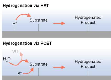
Fig. 4 Electricity-driven hydrogenation *via* hydrogen atom transfer (top) or proton-coupled electron transfer (bottom) processes.<sup>97</sup>
