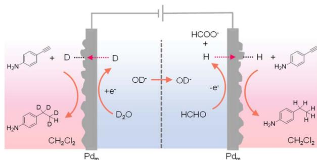
Fig. 14 A four-compartment assembly for the hydrogenation of 4-ethynylaniline in the chamber outside of the anode chamber coupled with its deuteration in a chamber next to the cathode chamber.<sup>150</sup>
