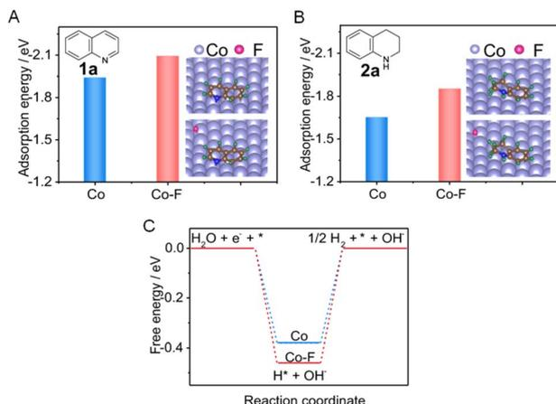
Fig. 8 (A and B) Comparisons of adsorption energies of **1a** and **2a** on pure Co (A) and Co-F (B), respectively (inset: the stable adsorption configurations of **1a** and **2a**). (C) The calculated free energy for H<sup>\*</sup> formation on Co versus CoF. This figure has been adapted/reproduced from ref. 112 with permission from Nature Publishing Group, copyright 2022.
