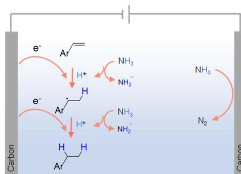
Fig. 3 Possible mechanism for the electrochemical hydrogenation of olefins using NH<sub>3</sub> as the hydrogen source using 0.1 M LiClO<sub>4</sub> in CH<sub>3</sub>CN as the electrolyte with NH<sub>3</sub> (1 atm) as the nitrogen source.<sup>83</sup>
