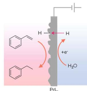
Fig. 13 Hydrogenation of styrene to ethylbenzene using a Pd sheet electrode.<sup>137</sup>
