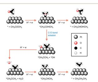
Fig. 6 The most favourable reaction pathways computed for acetone reduction to 2-propanol and propane at Pt electrodes. 105
