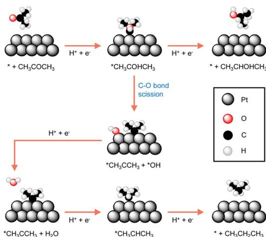
Fig. 6 The most favourable reaction pathways computed for acetone reduction to 2-propanol and propane at Pt electrodes.<sup>105</sup>
