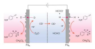
Fig. 14 A four-compartment assembly for the hydrogenation of 4-ethynylaniline in the chamber outside of the anode chamber coupled with its deuteration in a chamber next to the cathode chamber.<sup>150</sup>
