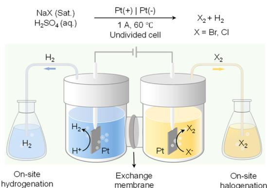
Fig. 12 Paired electrolysis consisting of on-site hydrogenation coupled with on-site halogenation (X: Br or Cl).<sup>136</sup>
