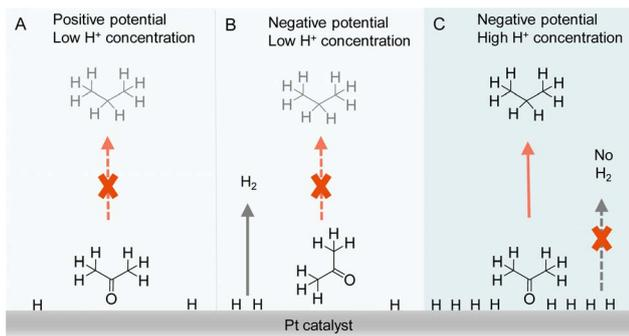
Fig. 10 Representations of acetone to propane hydrogenation (A) under positive potential in electrolyte with low  $H^+$  (0.1 M  $H_2SO_4$ ) concentration, (B) under negative potential in electrolyte with low  $H^+$  (0.1 M  $H_2SO_4$ ) concentration, and (C) under negative potential in electrolyte with high  $H^+$  (1 M  $H_2SO_4$ ) concentration.<sup>122</sup>
