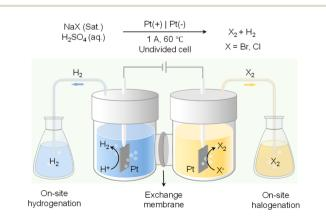
Fig. 12 Paired electrolysis consisting of on-site hydrogenation coupled with on-site halogenation (X: Br or CI).  $^{136}$
