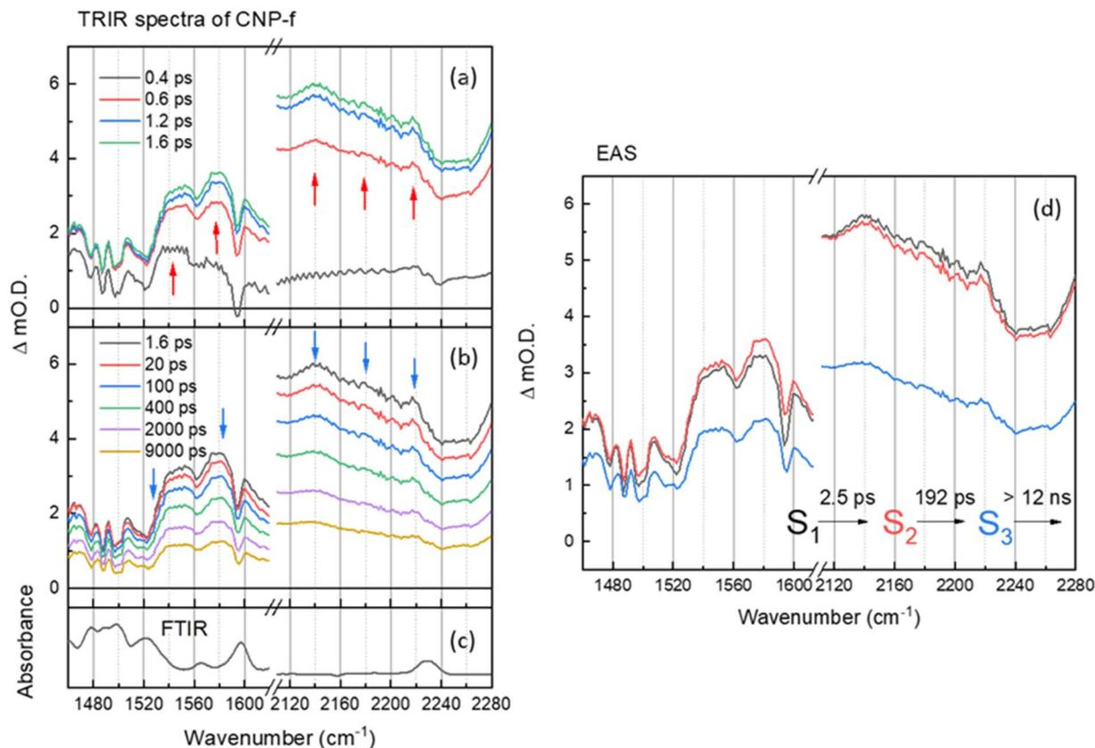
Fig. 3 (a and b) ps–ns time-resolved infrared (TRIR) spectra of CNP-f films of the aromatic C=C and CN spectral regions following excitation at 380 nm, shown at different time delays. The arrows show the direction of the spectral evolution (c) the FTIR spectra CNP-f. (d) The corresponding evolution associated spectra (EAS) and time constants generated through 3 compartment sequential pathway global lifetime analysis (GLA) of data in part (a and b).
