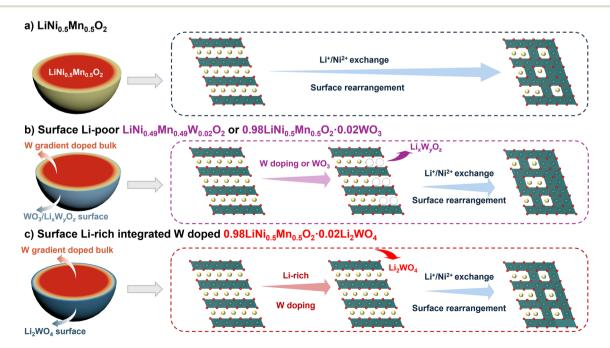
Fig. 6 Schematic diagram for the mechanism of  $LiNi_{0.5}Mn_{0.5}O_2$  (a), surface Li-poor  $LiNi_{0.49}Mn_{0.49}W_{0.02}O_2$  or  $0.98LiNi_{0.5}Mn_{0.5}O_2 \cdot 0.02WO_3$  (b) and surface Li-enriched  $0.98LiNi_{0.5}Mn_{0.5}O_2 \cdot 0.02Li_2WO_4$  (c) during delithiation.
