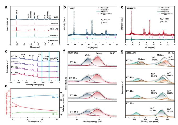
Fig. 1 (a) XRD pattern of NM50, NM50-W2, NM50-LW2, and NM50-W02; (b and c) Rietveld refinements of the XRD pattern of NM50 (b) and NM50-LW2 (c). (d) XPS full spectrum of NM50-LW2 obtained with different etching times; (e) relative content of Ni, Mn and W elements obtained by XPS with different etching times; (f and g) XPS depth profiles of W 4f (f) and Mn 2p (g) with different etching times.
