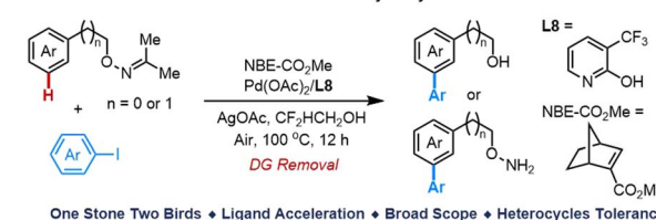
Scheme 1 meta -C–H functionalization of alcohol and hydroxylamine via Pd/NBE relay catalysis.
