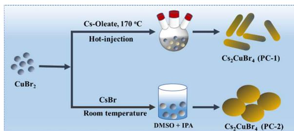
Scheme 1 Schematic representation showing the structural modulation of Cs<sub>2</sub>CuBr<sub>4</sub> by two different synthesis methods: (i) hot-injection (PC-1) and (ii) room temperature (PC-2).
