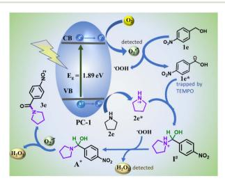
Scheme 2 The proposed mechanism for photocatalytic oxidative amidation of alcohol is based on the detected intermediates.
