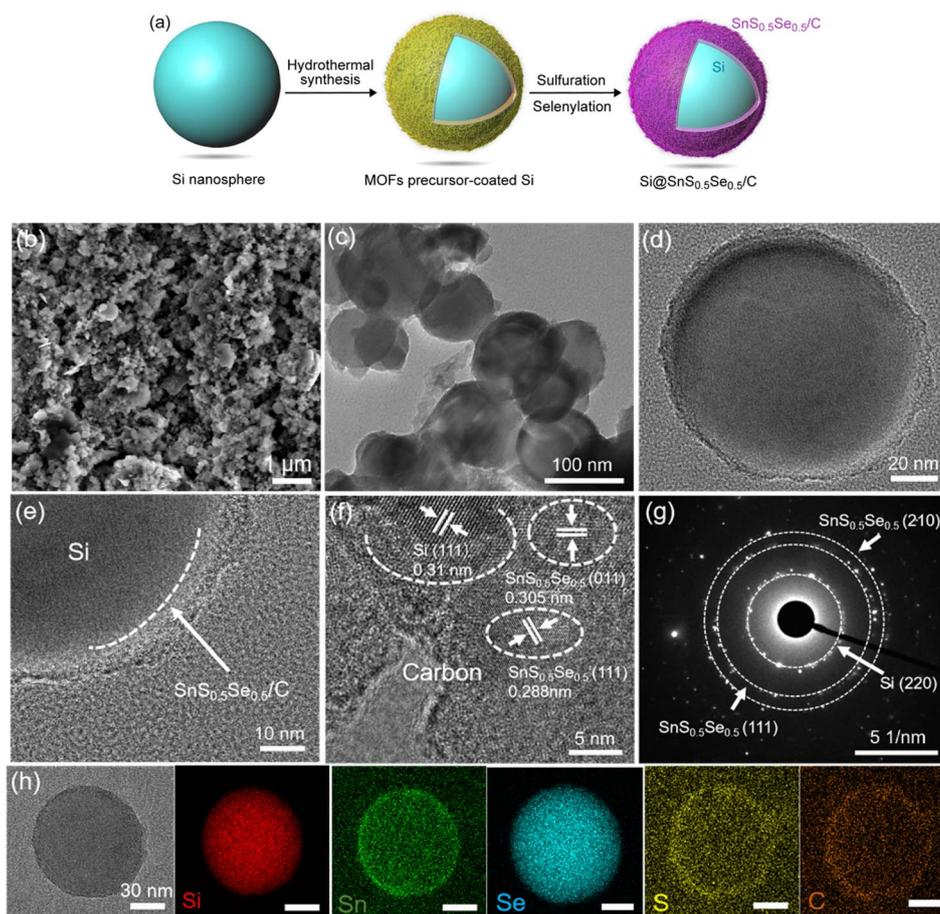
Fig. 1 (a) Illustration of the preparation of Si@SnS<sub>0.5</sub>Se<sub>0.5</sub>/C hybrid nanospheres. (b) SEM image of Si@SnS<sub>0.5</sub>Se<sub>0.5</sub>/C. (c–e) TEM and (f) HRTEM photographs, (g) corresponding SAED pattern, and (h) TEM photograph and mappings of Si@SnS<sub>0.5</sub>Se<sub>0.5</sub>/C.
