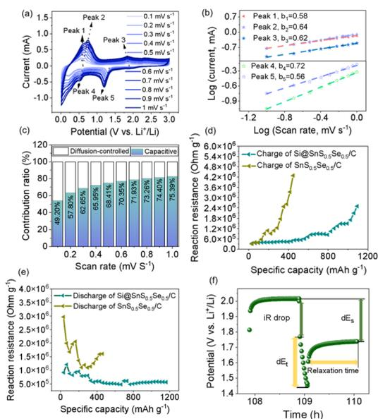
Fig. 4 (a) CV curves at 0.1 to 1.0 mV s<sup>-1</sup>. (b) Log(*i*) vs. log(*v*) of the oxidization and reduction peaks, and (c) ratio of the contributions. *In situ* reaction impedances of Si@Sn<sub>0.5</sub>Se<sub>0.5</sub>/C and Sn<sub>0.5</sub>Se<sub>0.5</sub>/C during (d) discharge and (e) charge. (f) Illustration of  $dE_s$ ,  $dE_t$ , and the *iR* drop.
