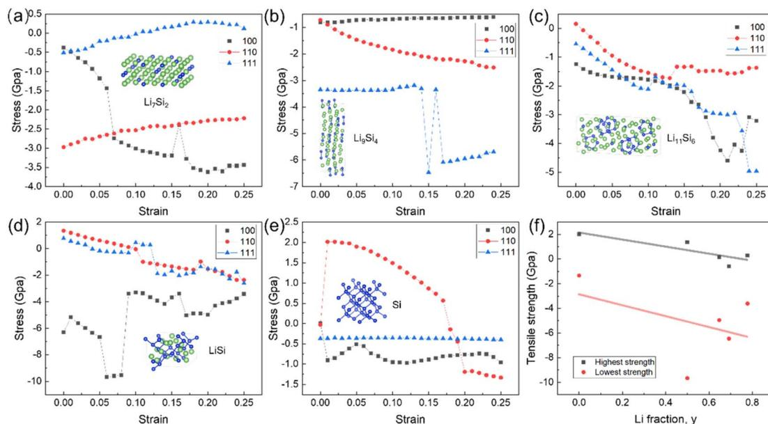
Fig. 5 The relationships of stress and strain in the Li–Si system with different Li and Si ratios: (a)  $\text{Li}_7\text{Si}_2$ , (b)  $\text{Li}_9\text{Si}_4$ , (c)  $\text{Li}_{11}\text{Si}_6$ , (d)  $\text{LiSi}$ , and (e)  $\text{Si}$ . The crystal structure was inserted in each figure. The green and blue spheres represent Li and Si atoms, respectively. (f) Relationships between maximum and minimum principal stress and the Li fraction.
