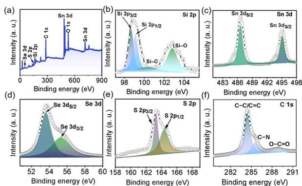
Fig. 2 (a) XPS survey spectrum of Si@SnS<sub>0.5</sub>Se<sub>0.5</sub>/C. XPS spectra of (b) Si 2p, (c) Sn 3d, (d) Se 3d, (e) S 2p, and (f) C 1s.
