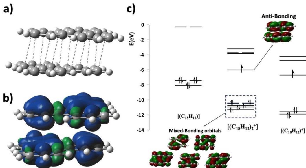
Fig. 7 (a) Optimized structure of the mono-cationic TP dimer,  $[(C_{18}H_{12})_2]^+$ , with dashed lines highlighting short C...C contacts. (b) Spin density of  $[(C_{18}H_{12})_2]^+$ . (c) Molecular orbital (MO) diagram for  $[(C_{18}H_{12})_2]^+$ , showing ten valence orbitals derived from the combination of five valence orbitals each from the neutral and cationic triphenylene monomers. Spin density is plotted using  $|iso| = 0.0008$  and orbitals are plotted using  $|iso| = 0.015$ .
