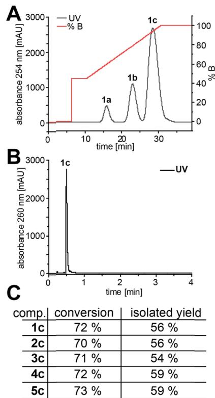
Fig. 3 Purification and purity of preparative EbPPK2 reactions (10 μmol). (A) Chromatogram of the anion exchange chromatography exemplified for **1c** (for **2c–5c** see Fig. S45†). Performed on an ÄKTA purifier. Buffer A: ddH<sub>2</sub>O; buffer B: 100 mM NaClO<sub>4</sub>, pH 4.2. (B) Chromatogram of the LC-MS analysis of ATP (**1c**). The corresponding chromatograms and EIC for **1c–5c** can be found in Fig. S46–S50.† (C) Conversion and isolated yield for **1c–5c**.
