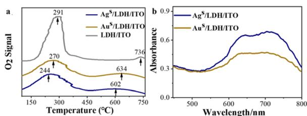
Fig. 4 (a) O<sub>2</sub>-TPD pattern of LDH/ITO, Au<sup>s</sup>/LDH/ITO and Ag<sup>s</sup>/LDH/ITO electrodes; (b) UV-vis spectra of methyl hydrazone for the Ag<sup>s</sup>/LDH/ITO and Au<sup>s</sup>/LDH/ITO electrodes in KOH/DMSO solution.
