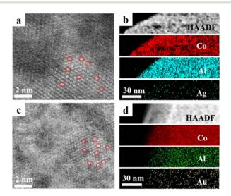
Fig. 2 (a) HAADF-STEM image and (b) STEM-EDS mapping images of Co, Al, and Ag for Ag<sup>s</sup>/LDH/ITO; (c) HAADF-STEM image and (d) STEM-EDS mapping images of Co, Al, and Au for Au<sup>s</sup>/LDH/ITO.
