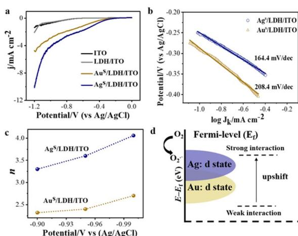
Fig. 5 (a) Current density ( $j$ )–voltage curves in O<sub>2</sub>-saturated PBS (pH = 7.5) at ITO, LDH/ITO, Au<sup>s</sup>/LDH/ITO and Ag<sup>s</sup>/LDH/ITO electrodes; (b) Tafel slope curves of Ag<sup>s</sup>/LDH/ITO and Au<sup>s</sup>/LDH/ITO electrodes; (c) average electron transfer numbers ( $n$ ) calculated from the K–L equation during the oxygen reduction reaction; (d) schematic illustration of the d-band center shift from the Fermi level for single atomic Ag and Au.
