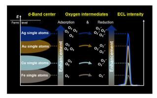
**Scheme 1** Schematic illustration of ECL to spot the positions of dband centers of single-atom catalysts.
