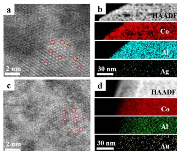
Fig. 2 (a) HAADF-STEM image and (b) STEM-EDS mapping images of Co, Al, and Ag for  $\text{Ag}^{\text{s}}/\text{LDH}/\text{ITO}$ ; (c) HAADF-STEM image and (d) STEM-EDS mapping images of Co, Al, and Au for  $\text{Au}^{\text{s}}/\text{LDH}/\text{ITO}$ .
