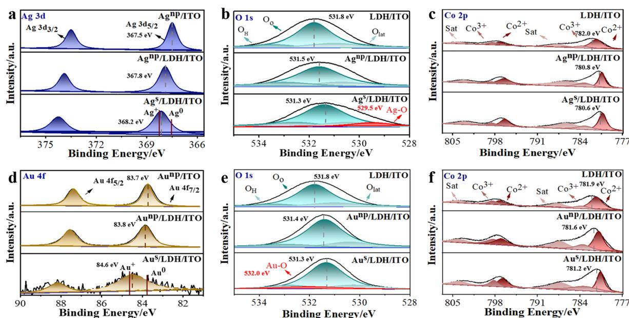
Fig. 3 High-resolution XPS spectra of (a) Ag 3d, (b) O 1s and (c) Co 2p for LDH/ITO, Ag<sup>NP</sup>/ITO, Ag<sup>NP</sup>/LDH/ITO and Ag<sup>S</sup>/LDH/ITO; high-resolution XPS spectra of (d) Au 4f, (e) O 1s and (f) Co 2p for LDH/ITO, Au<sup>NP</sup>/ITO, Au<sup>NP</sup>/LDH/ITO and Au<sup>S</sup>/LDH/ITO (the positions of the dotted line are marked in the diagram).
